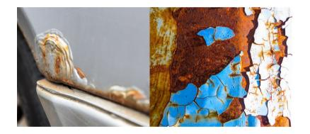
Improper surface preparation of metal surfaces with oxidation leads to immediate paint failure. This can present as peeling, bubbling, or flaking of the coating. Proper preparation will enhance adhesion and significantly reduce the possibility of coating failure.
