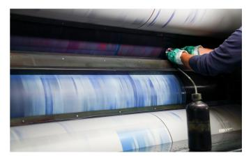
Aerogreen 4175 is shown being used on the roller drum. The picture on the left demonstrates the system being flushed with the diluted cleaning solution. The picture on the right demonstrates how to gently wipe down the surfaces, paying particular attention to the areas that come into direct contact with the coating. It is advisable to consult the application guidelines for optimal results.
